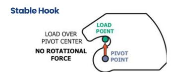
The hook on the left above is SSI's stable hook design. It can be seen that the lift point of the hook (represented by the green dot) is directly above the pivot point of the hook (represented by the blue dot) this creates No Rotational Force on the hook when the hook is under load.
