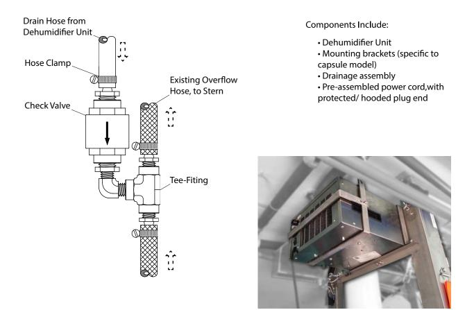
ESK's are SSI's engineered packages of additional components (or modified components) to "add-on" to your existing SSI offshore capsule. The goal of these kits is to offer additional functionality, ease of operation and ultimately added safety to your Survival Systems International Capsule. Since SSI is the OEM of your lifeboat (capsule), as well as the designer and manufacturer of these Enhanced Safety Kits, the installation process is seemless and cost effective.
