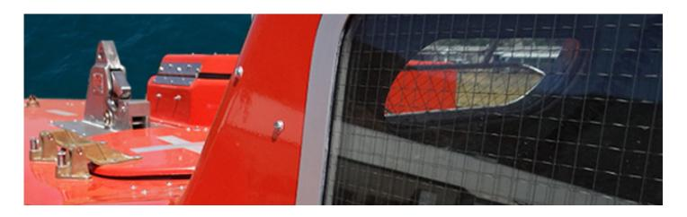
With a twin-fall capsule this job needs to be performed by two individuals. The access to the hook up is usually far more awkward than shown in the capsule above. Additionally it should be noted that involving two individuals doubles the danger of an incorrect hook up.
